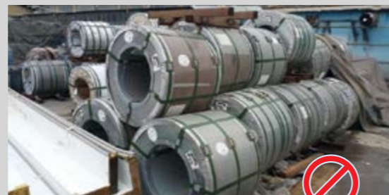
▲ Incorrect outdoor storage (cover not used)
